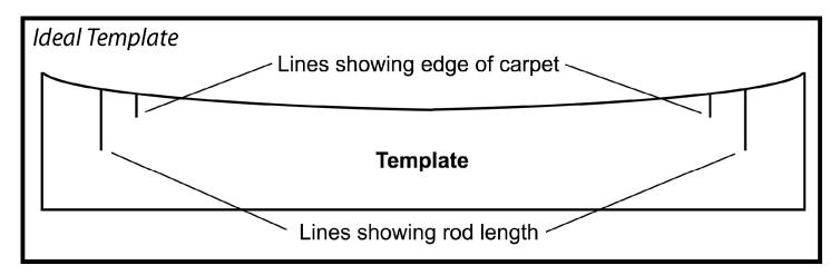
If you are making the template on an uncarpeted stair, bear in mind that the rods lies approximately 14mm from the riser with carpet and gripper behind it. Therefore your pencil point should be 14mm from the riser when putting its mark on the template.
